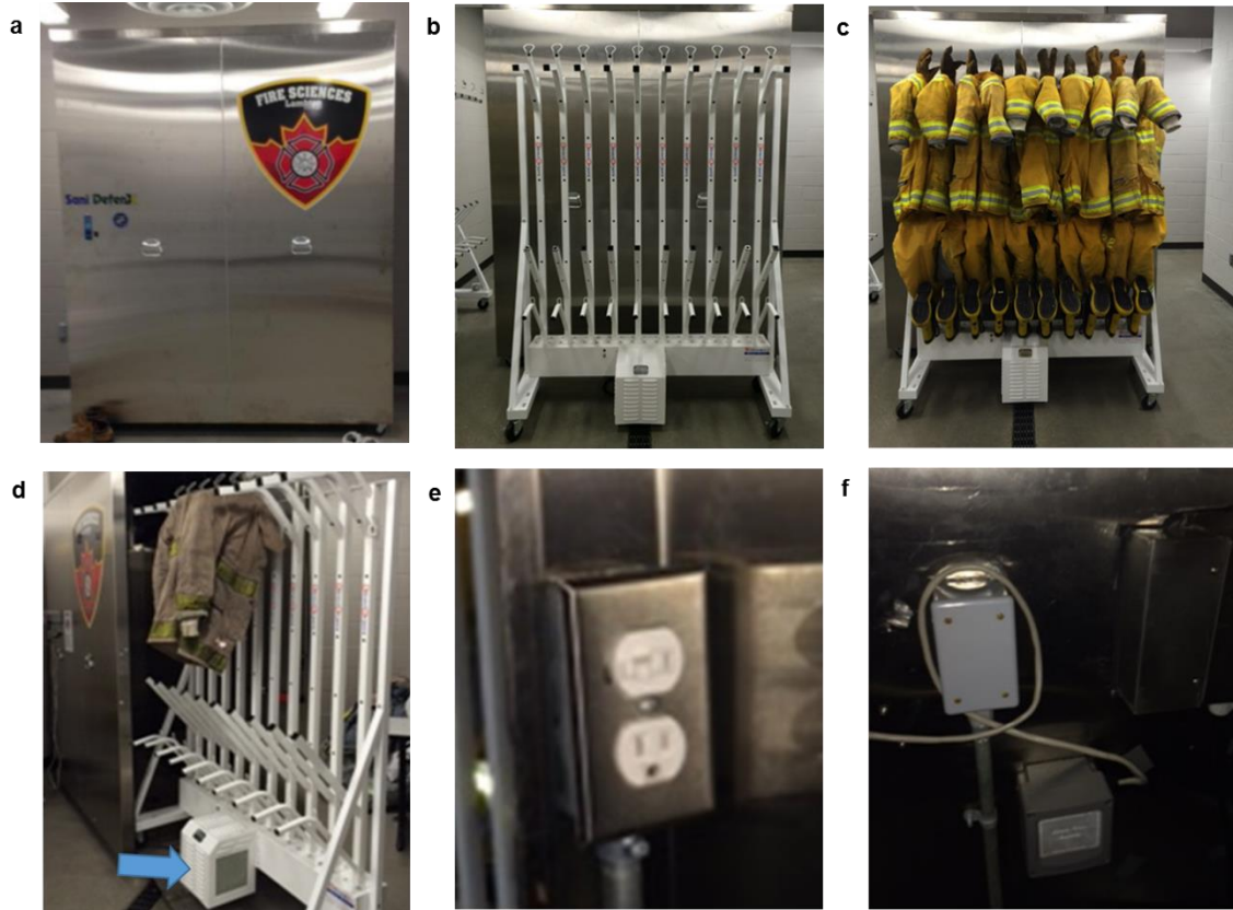
Fig. 2. Sani Sport cabinet for sanitization of Firefighters Turnout Gear. a) Prototype of a cabinet in Lambton College School of Fire Sciences and Public Safety. b) Empty Gear drying rack. c) “Full load”, rack loaded with five Gear sets each comprising jacket, pants, helmet, boots, and gloves. d) “Single load”, rack loaded with one jacket (arrow points to fan activated when the rack is plugged into the mains). e) Plug-in for the rack inside of the cabinet. f) Electrical assembly for the plug inside of the cabinet.
